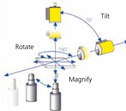
Under any combination of rotate, tilt and magnification, true concentric imaging ensures that the region of interest remains completely locked into the center of the field of view.
