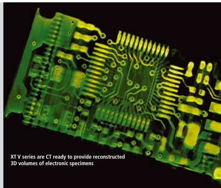
XT V series are CT ready to provide reconstructed 3D volumes of electronic specimens
