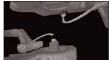
Damaged wirebond in IC
